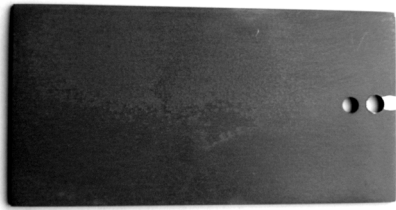
图 2 配方 1 制备的硬质阳极氧化膜 Fig. 2 Hard anodic coating prepared by formula 1
