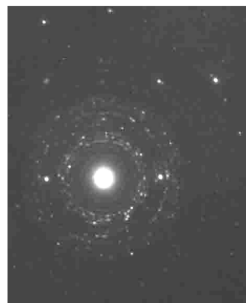
图 4 A 区电子衍射花样 Fig. 4 The electron diffraction diagram of part A
