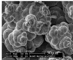
图 3 复合镀层表面形貌 1 000 × Figure 3 Surface morphology of the composite coating 1 000 ×
