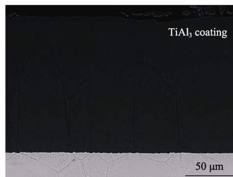
图 5 钛基合金渗铝后的截面形貌<sup>[21]</sup>Fig.5 Cross-sectional morphology of aluminide coating on Ti-based alloy<sup>[21]</sup>
