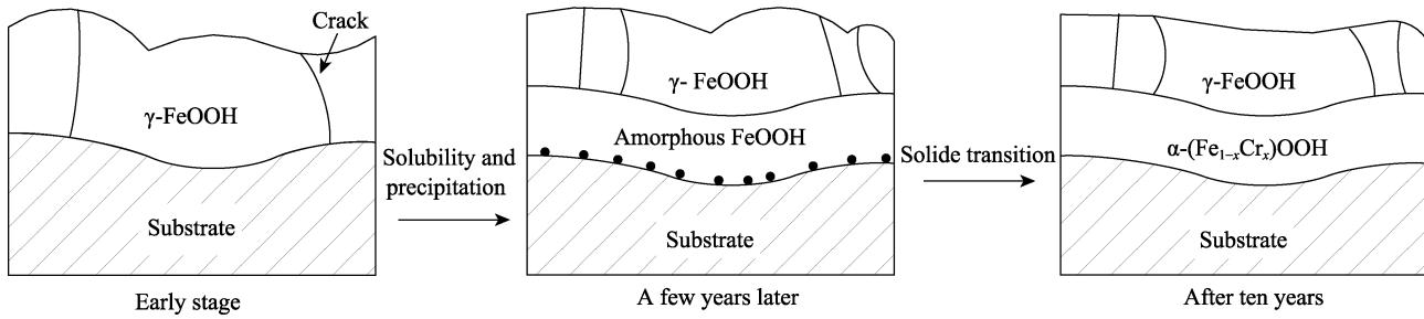
图2 耐候钢锈层的形成过程<sup>[29-30]</sup>Fig.2 Growth process of rust layer on weathering steel<sup>[29-30]</sup>
