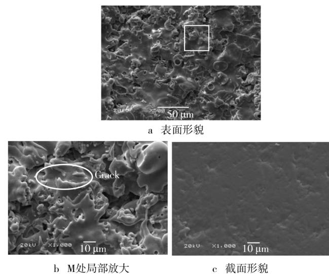
图 5 纳米  $\text{Al}_2\text{O}_3$  涂层微观形貌(SEM)Fig. 5 Micrographs of nano  $\text{Al}_2\text{O}_3$  coatings: a) surface morphology; b) magnification of M; c) cross-section morphology (SEM)
